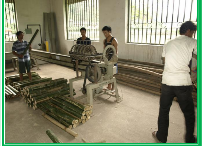
Practice on Radial Splitting Machine
