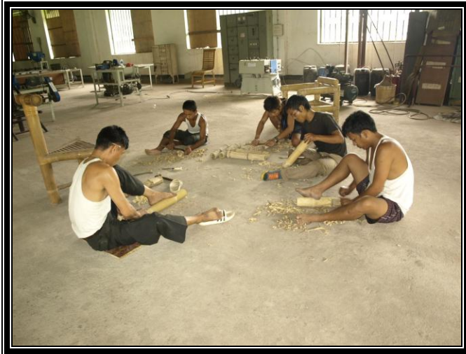
Raw material preparation for furniture
