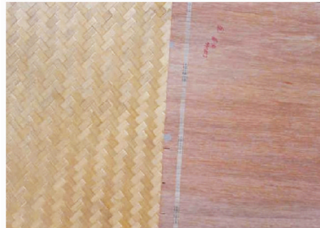
Fig. 2.2.2.1. Bamboo mat veneer composite.
