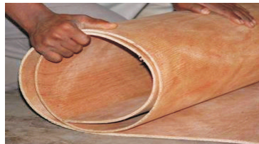
Fig. 2.2.10.1. Flexi-ply with bamboo mat as core.
