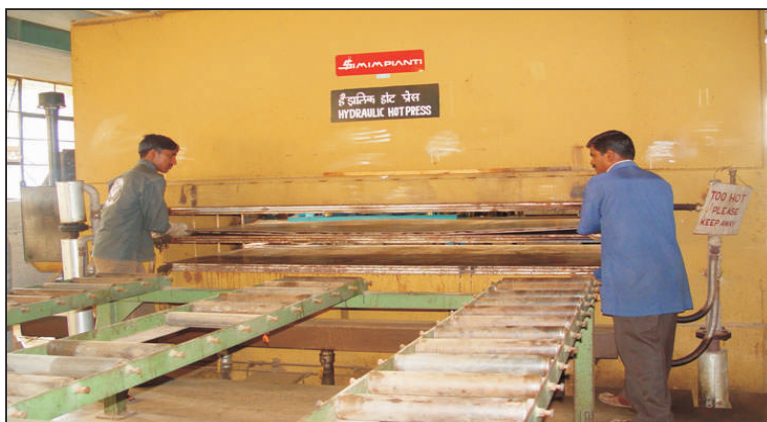
Fig. 2.2. Pilot plant in IPIRTI for manufacture of bamboo mat board (2.44 m × 1.22 m size).
