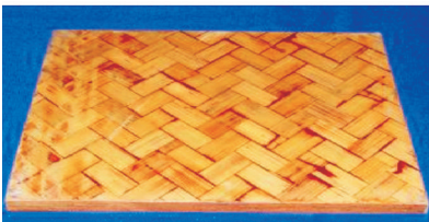
Fig. 2.2.9.1. High density shuttering grade BMB.
