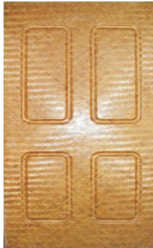
Fig. 2.2.8.1. Bamboo mat moulded skin board.
